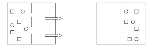
Filtration can be achieved through either increasing the pressure on the blood side of the filter or increasing the negative pressure on the dialysate side of the filter. (Whitaker in Clochsey et al 1996:936)
